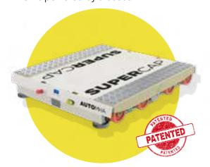
**Supercap ES**: the **satellite** on board the parent shuttle, which performs pallet storage and retrieval operations in the storage lanes based on commands issued via WI-FI from the Mover shuttle.
