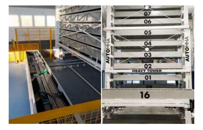
HeavyTower can be configured as an inter-operational buffer and used alongside cutting and production machines. Automha's HeavyTower is the ideal solution for storing steel bars and profiles, tubes, heavy accessories, semi-processed items, parts, molds and large items in general.
