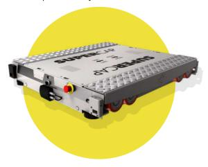
**Supercap ES**: the **satellite** on board the parent shuttle, which performs pallet storage and retrieval operations in the storage lanes based on commands issued via WI-FI from the Mover shuttle.
